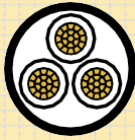
Construction of 3 core cable
