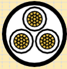
Construction of 3 core cable
